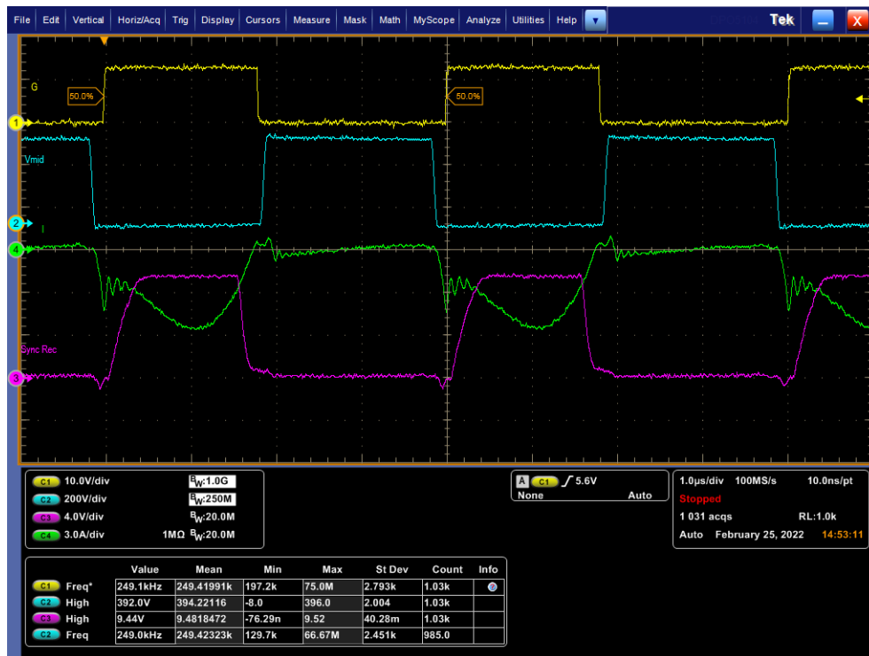
Figure 11 - LLC Eval Operating at 100 W. 1 \mu s/div.
